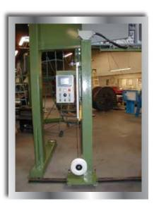
**Dancers** are primarily used for speed regulation of winding or unwinding equipment. They can act as the primary mode of regulation, or as a trim to another speed reference. They can be linear or pivoting for inline applications, or articulating for applications whereby the product requires a fleeting angle entrance to the process centerline. They are usually used in slower line speed applications.
